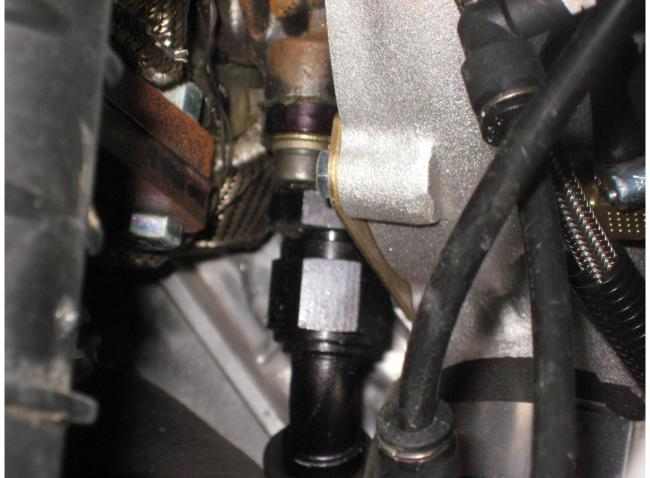
23. Next your going to want to run the oil feed line. There's a supplied brass T fitting that your going to use on the oil filter housing. Remove the oil pressure sensor and install the T fitting, then install the oil pressure sensor into the T fitting and the new -4 AN oil feed line. This feed line goes to the top side of the turbocharger. The braided steel line in the pictures is different then the push-lock hose supplied in the kit.
