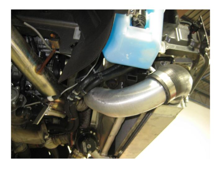
40. Supplied is a 45 degree silicon coupler, connect that to the pipe feeding up to the throttle body and then use the 90 degree aluminum pipe to connect to the intercooler as seen above.
