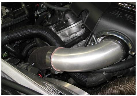
41. Following the diagram below set up the vacuum and boost references for the wastegates and blow off valves. Install a T into the brake boost line to get a vac/ boost reference.
